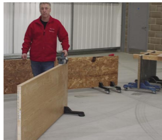
Gripped Dave Crampton is a joiner and developed his Magic Grippers because so many of his colleagues have problems holding doors for trimming and hinging, but the invention now has many other uses
